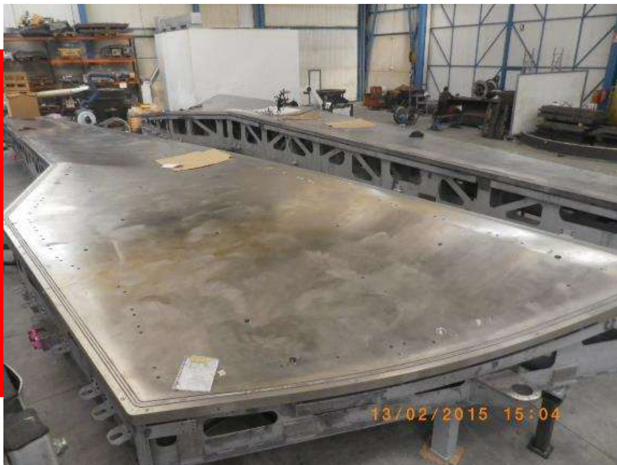
OML TOOLS for lay up and molding WING OF A220
